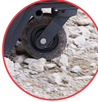
Wide drive and steer wheels—for reduced ground pressure and increased traction on tough job sites.
