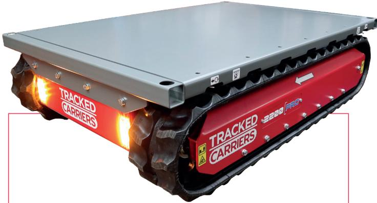
The 2200 series from Tracked Carriers offers an unrivalled method of transporting heavy goods through confined spaces. Only 950mm wide, the 2200 R and 2200 PRO models are heavyweights in compact packaging.
